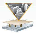
Conventional abrasive grain tends to "plow" through the metal, causing heat to build up in the workpiece and the abrasive — resulting in a slower, less consistent cut and shorter disc life.
